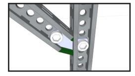
4b 45 degree connection exploded side-view.
